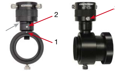
To use the pick-up prism of the Baader Off Axis Guider for RCC (left) or of older Celestron Radial Guiders, you first need to remove the T-2-sleeve by opening screw 1. Now loosen the the screws 2 to remove the spacer ring (grey arrow), and reattach the prism unit again at the eyepiece clamp. Screw 3 is used to tilt the prism.
