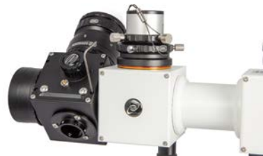
The orientation of the adapter threads on both sides can be changed with the four grub screws. This way, you can align instruments like the DADOS spectrograph in this image to the BFM II, or you can rotate the whole BFM, if it is screwed directly to the telescope.
