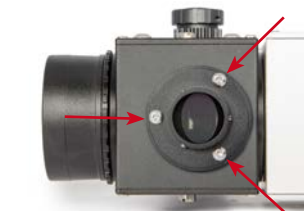
The screws for adjusting the bottom port of the BFM II.
