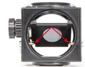
The two pins on which the mirror lays on
