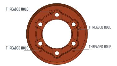
Note that this cover plate has four threaded holes for mounting the focus motor.
